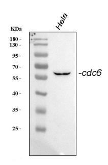
Western blot analysis of CDC6 using anti-CDC6 antibody (BA2581-2). The sample well of each lane was loaded with 30 ug of sample under reducing conditions.
