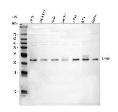
Western blot analysis of RAB11A using anti-RAB11A antibody (PB0836). The sample well of each lane was loaded with 30 ug of sample under reducing conditions.
